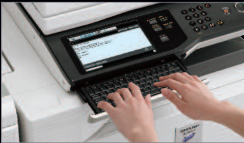
Standard retractable keyboard makes data entry quick and easy (N models only).
